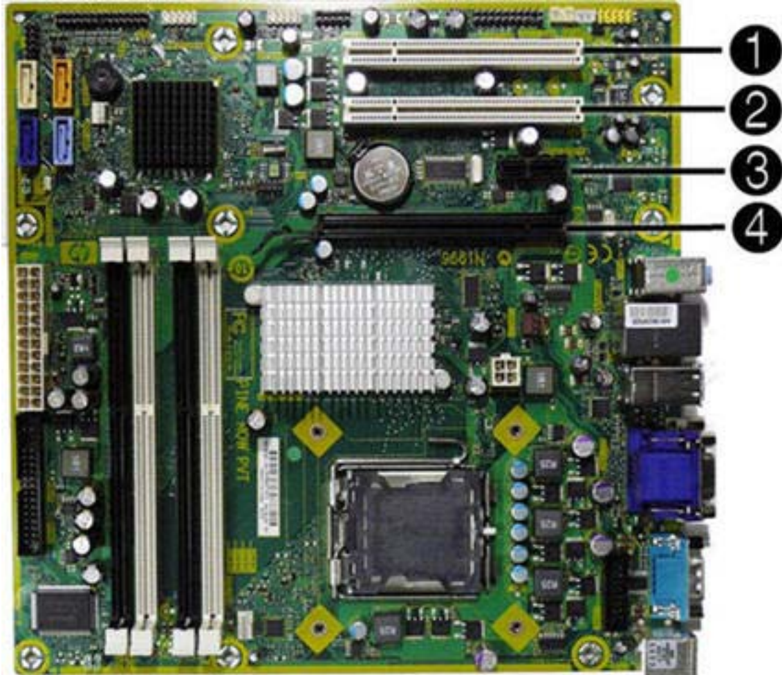
Figure 7-8 Expansion Slot Locations – HP Pro 3000/3080
